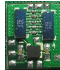
Parallel loop 2 (0.2nH) 9mm*9mm
